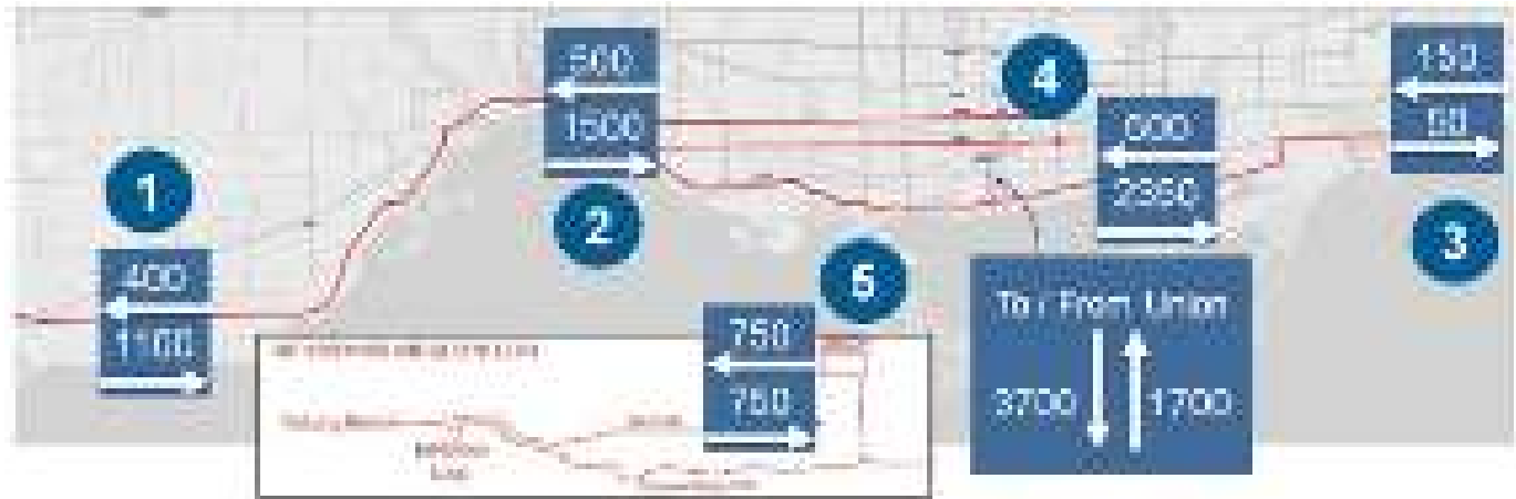
Figure 23: Summary 2041 Forecasted Transit Network Demand (AM Peak Hour) (Source: City of Toronto)
